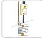
Equipment must be grounded correctly.
